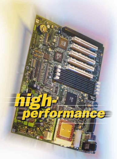
Alpha motherboards are designed to use standard PC components such as synchronous DRAM (SDRAM) DIMMs, PCI option cards, power supplies, and enclosures. The AlphaPC 164RX offers PCI and ISA slots, onboard PCI IDE, onboard Ethernet, and memory support for up to 512 MB of SDRAM in an ATX form factor.
