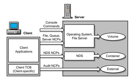
Figure 1-6 shows the architecture of the client and server software used by an auditor to perform audit processing. There are no server-based utilities for processing the server's audit trails; instead, auditors use client-based utilities (such as AUDITCON) to review audit trails and to display selected audit events.
