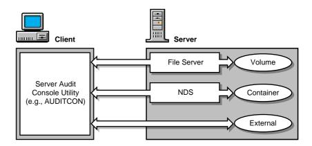
As shown in Figure 1-5, protected code in the server generates audit events to audit trails protected by the server. The operating system records console commands in volume SYS: audit trail.
