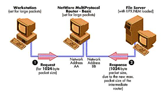
Figure 2: By allowing the NetWare packet size to be increased, LIP enhances the throughput over bridges and routers.
