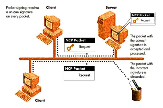
Figure 5: NCP Packet Signature prevents packet forging by requiring the client and server to sign each packet.
