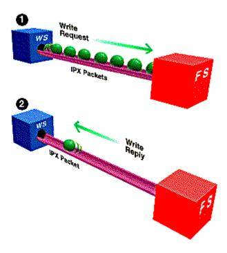
Figure 1: With Packet Burst, clients can have the server read or write large blocks of data comprising multiple packets.
