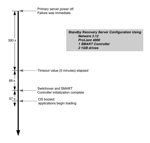
Figure 4: In this example of an automated switchover event, the recorded elapsed time—from failure of the primary server through loading of the operating system on the standby server—totaled 445 seconds (less than 7½ minutes). Additional time is needed for loading the applications being used and for client log on.
