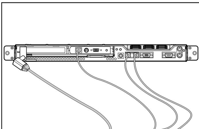
**Figure 10: Typical cabling using the Remote Insight Lights-Out Edition (DL360 shown)**
