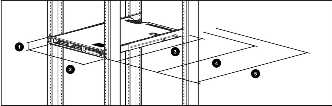
Figure 5: Dimension requirements for the Compaq Third-Party Rack Option Kit
