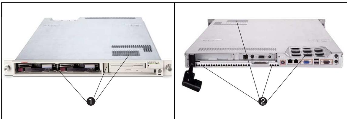
Figure 7: Intake ❶ and Exhaust ❷ vents for the ProLiant DL360 server
