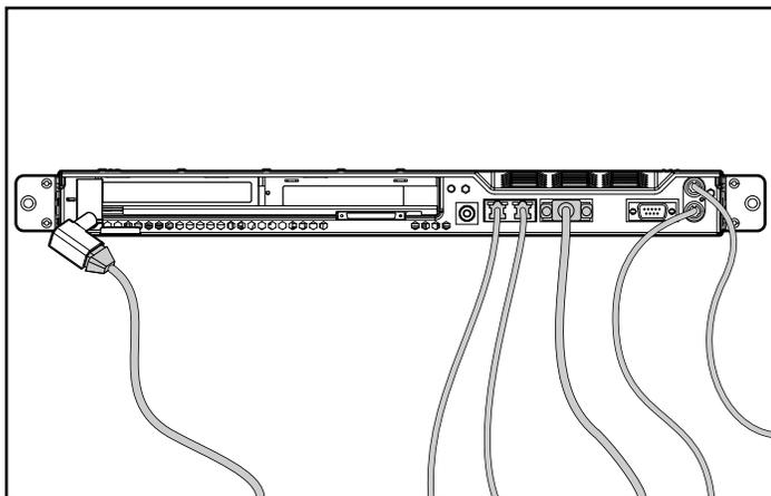
Figure 11: Typical cabling using server console switches (DL360 shown)
