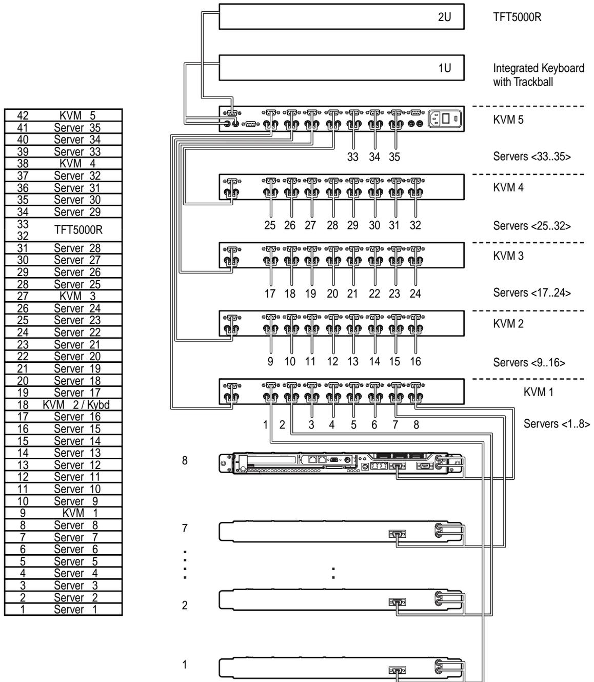
Figure 12: Typical KVM and cascading console switch solution for 35 ProLiant Servers
