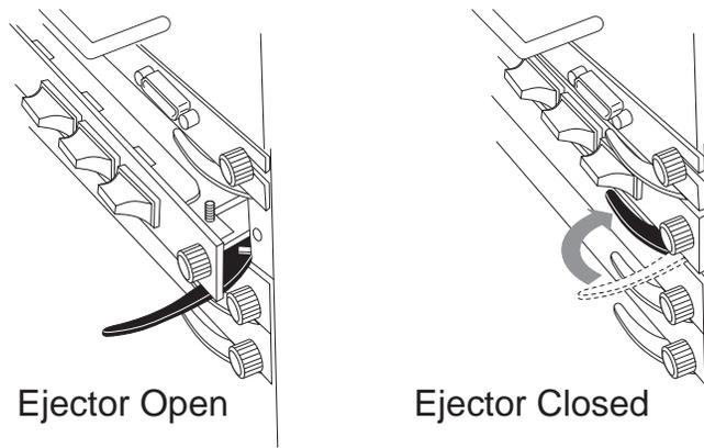
5 Tighten the black captive screws on the module.
