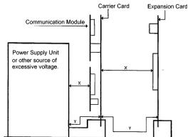
Except for the edge connector which plugs into the host's expansion slot, clearance distance (Xmm) and creepage distance (Ymm) as given in the above table, must be maintained between the communication card and any other assemblies which use or generate a hazardous voltage.
