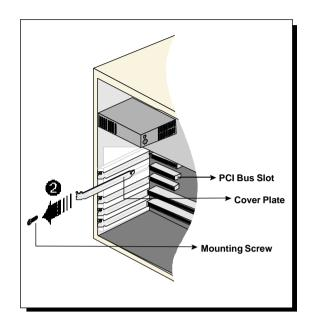
**3.** Align your card with the selected PCI Bus slot and firmly push it into the slot. If the card does not slide in, do not force it. Make sure that the card is lined up properly and try again.
