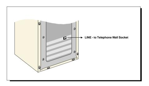
Connect one end of the **telephone extension cord** to the modem card and the other end to the **telephone wall socket**.
