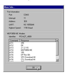
(If your modem is not installed properly, the set of AT commands will not be listed. You may also be prompted by an error message, stating that it was unable to open the COM Port. If this happens, refer to the *Appendix A - Frequently Asked Questions* "While testing the modem, the system gave an error message stating that it was unable to open the COM Port.")
