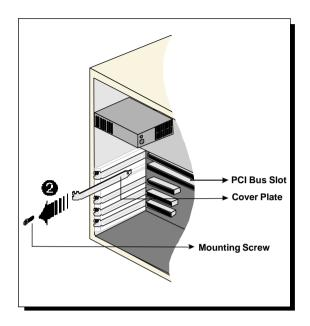
Align your card with the selected PCI Bus slot and firmly push it into the slot. If the card does not slide in, do not force it. Make sure that the card is lined up properly and try again.
