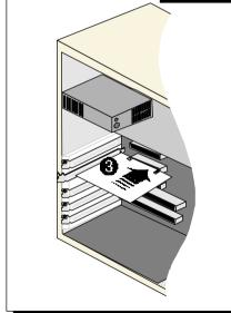
Align your card with the selected PCI Bus slot and firmly push it into the slot. If the card does not slide in, do not force it. Make sure that the card is aligned properly and try again.
