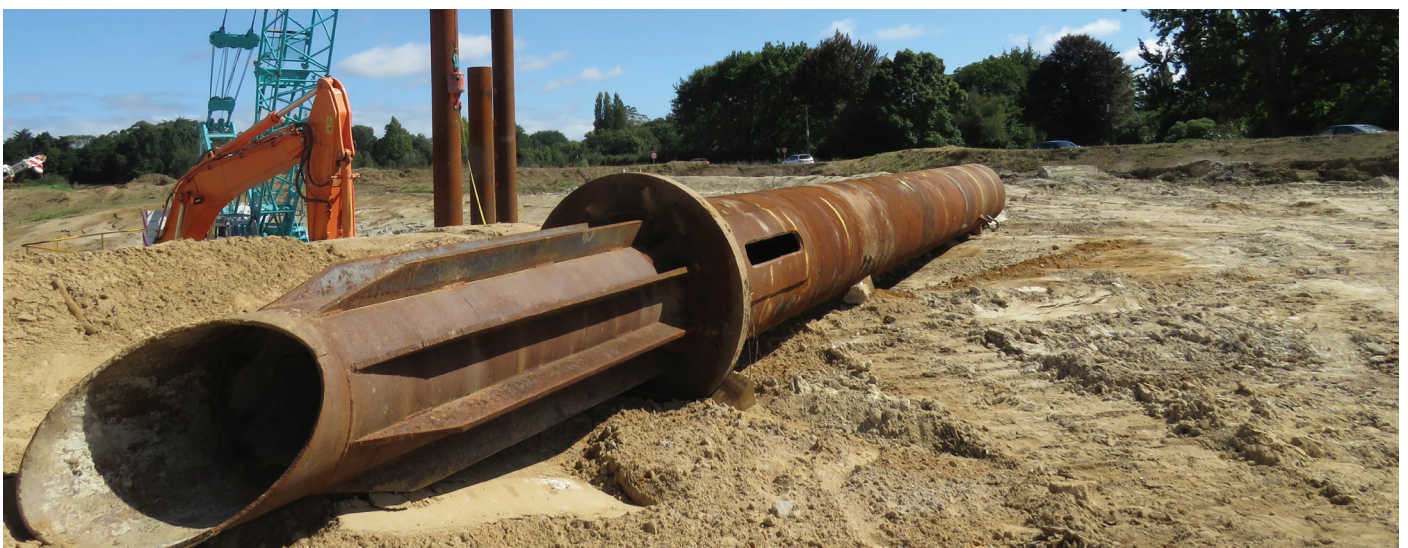
This driving dolly is used to test piles when they achieve their target depth
