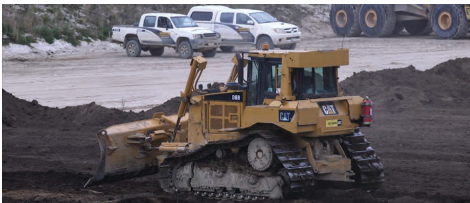
A bulldozer spreads topsoil to restore an area where sand has been extracted.
