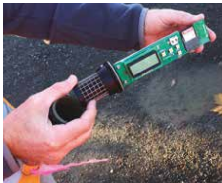
The echo-location calls of long-tailed bats have a distinct ultrasound frequency that can be measured by devices called acoustic bat monitors (ABMs). The ABMs record ultrasound calls on to an SD memory card which records and sorts the sounds by frequency.
