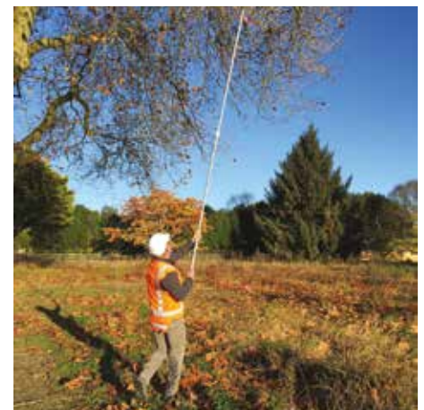
Monitoring devices are placed in trees using long poles
