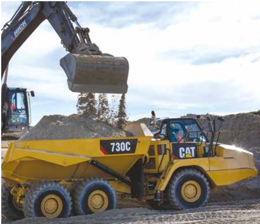
These earthmoving trucks are 6WD and can weigh up to 60 tonnes fully loaded.
