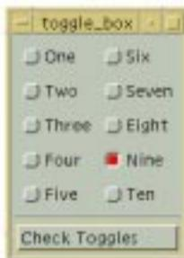
Figure 12-8: Output of the `toggle_box` program with `XmNradioBehavior` set True
