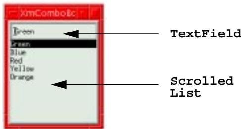
Figure 14-1: A ComboBox widget with the List permanently visible
