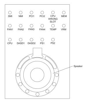
To replace the diagnostics panel LEDs, you must replace the interior LED and speaker assembly (see "Interior LED and speaker assembly" on page 212).
