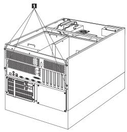
a. Loosen the screws 1 on the back of the shuttle; then, slide the shuttle to the rear of the system.
