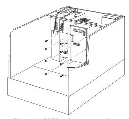
a. Remove the DASD backplane screws; then, remove the DASD backplane.
