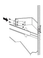
Installing the server in the rack: You will use eight screws (M4 by 8).
