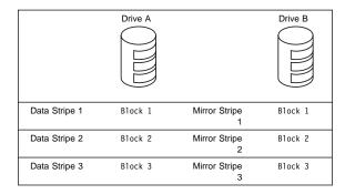
If one of the hard disk drives fails, the ServeRAID controller switches read and write requests to the remaining functional drive in the array.
