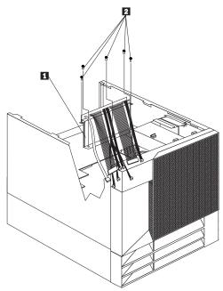
a. Remove the 5 power backplane screws 2 on the two top tabs and across the bottom front flange of the power backplane; then, remove the power backplane.
