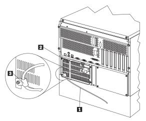
5. Plug the power cord into a properly grounded electrical outlet.
