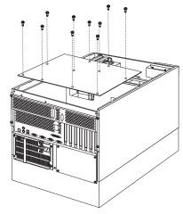
a. Remove the system board mounting screws; then, remove the system board.
