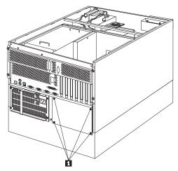
1. Remove the power supply filler panel screws **1**; then, remove the power supply filler panel.
