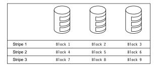
A hard disk failure within the array results in loss of data in the logical drive assigned RAID level-0, but *only in that logical drive*. If there are logical drives assigned RAID level-1 or level-5 in the same array, they will not lose data.
