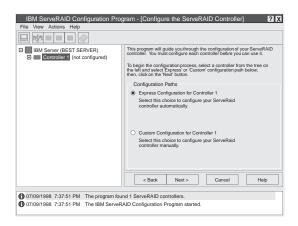
Select the **Cancel** button to switch from the Configuration mode to the Information mode. all ServeRAID controllers in the server are configured, the program starts in the Information mode and a screen similar to the following appears.
