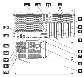
PCI Expansion Slots: The server has five peripheral component interconnect (PCI) expansion slots. Four of the PCI slots support hot-plug PCI adapters. The remaining, non-hot-plug PCI slot supports only a short adapter.
