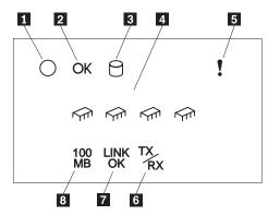
1 System Power Light: When this green light is on, system power is present in the server. When this light flashes, the server is in standby mode (the system power supply is turned off and ac current is present). When this light is off, either a power supply, ac power, or a light has failed.
