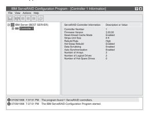
Select the icon on the Tool Bar to switch from the Information mode to the Configuration mode.
