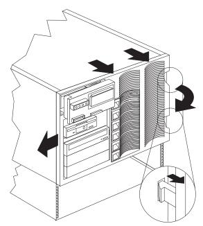
a. While releasing the side bezel tabs, rotate the right side of the bezel away from the system; then, unhook the left side bezel tabs.
