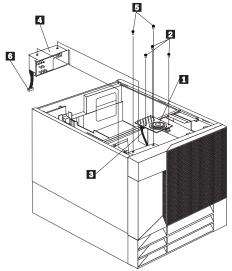
a. Remove the information LED panel assembly screws5; then, remove the assembly4.
