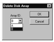
2. Select the desired disk array ID from the pull-down list.
