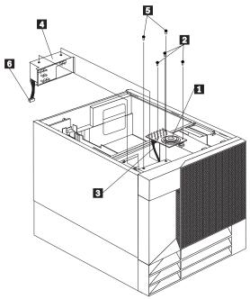
a. Remove the interior LED and speaker assembly mounting screws 2 . then; remove the interior LED and speaker assembly 1
