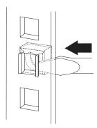
Attach a slide-bracket assembly to the front of the rack:
