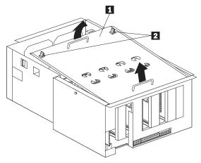
Processor support tray coverQuarter-turn fasteners
