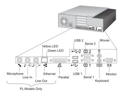
**Tower model:** The following illustration shows the location of the external connectors on the rear of the tower model.
