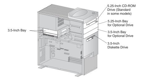
The PC 300GL tower model has six expansion slots. One or more of these slots might be occupied, depending on the model of your computer. Unoccupied slots can be used for installing adapters. The PC 300PL tower model has an additional AGP adapter expansion slot.
