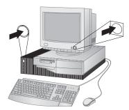
Turn on the monitor and other external devices first, and then turn on the computer. You see a logo screen while the computer performs a short self-test. Upon successful completion the logo screen disappears, the BIOS is loaded, and the software is loaded (in models with preinstalled software).
