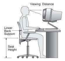
Adjust the monitor so the top of the screen is at, or slightly below, eye level. Place the monitor at a comfortable viewing distance, usually 51 to 61 cm (20 to 24 in.), and position it so you can view it without having to twist your body.
