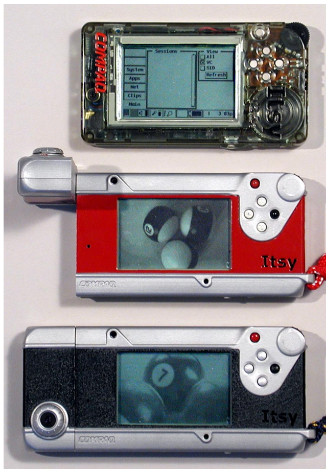
Figure 1: Three Itsy Pocket Computers. At the top of the picture is an unmodified Itsy. It is 118mm x 65mm x 16mm, and weighs (including battery) 130g with a molded plastic case. Below it are two units with the camera extension that are 147mm x 64mm x 20.5mm and weigh (including battery) 195g with a SLA epoxy case, or 267g with a NC tooled aluminum case.
