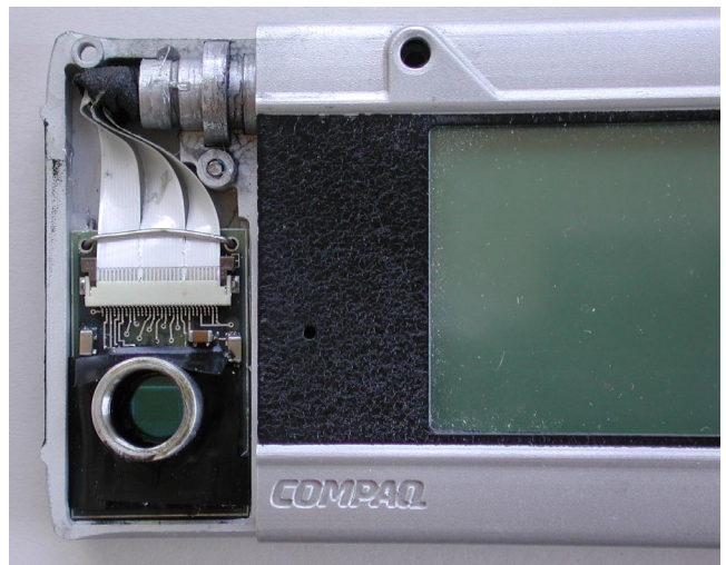
Figure 4: Itsy shown face up with the front of the image sensor case removed.
