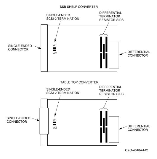
Figure 2–5 DWZZB–VW End-Bus Bus Terminators
