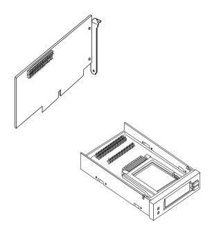
2 Hold the two connectors together tightly on the ribbon cable from Slot 2 on the card adapter and connect it to the 100-pin header on the ISA-bus host adapter labeled Slot 2. Make sure the two connectors are correctly aligned with the 100-pin header. Match pin 1 on the ribbon cable with pin 1 on the connector.
