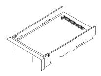
7 Secure the card adapter or mounting bracket to the PC chassis with four screws provided in your kit.
