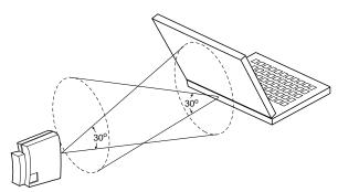
Be sure that both infrared devices are within this 30-degree cone. File transmission will fail if one of the devices is turned too far to the right or left or is much higher or lower than the other device.
