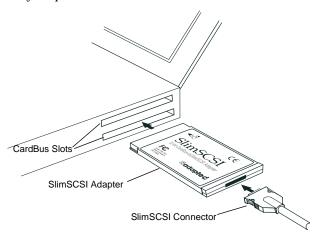
2 Plug the SCSI connector on the other end of the SlimSCSI cable into a SCSI device, as shown below:
