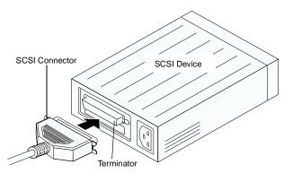
3 (Optional) Connect up to two additional SCSI devices by daisy-chaining them to the first device, as shown in the following diagram. (Additional cables are APA-1480 Installation Guide (OEM)
