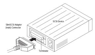
5 (Optional) Connect up to seven additional SCSI devices by daisy-chaining them as shown below. You need an additional external SCSI cable for each device:
