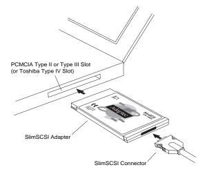
**3** Insert the SlimSCSI adapter in a PC Card (PCMCIA) Type II or Type III slot, or a Toshiba Type IV slot on your portable PC as shown above. Plug the 50-pin connector on the other end of the SlimSCSI cable into the first (or only) SCSI device, as shown below. The 50-pin low-density connector is shown here:
