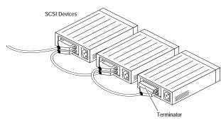
**6** Terminate the *last* (or *only*) SCSI device connected to the SlimSCSI adapter.
