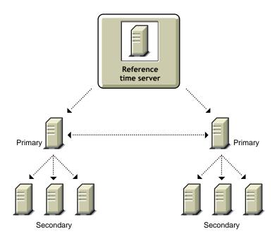
The following figure illustrates a network using an external time server that provides time to two Reference time servers, which are geographically distant.
