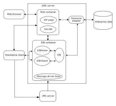
The following diagram illustrates how resource adapters can be used in J2EE applications.
