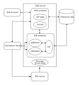
The following diagram shows how EJBs can be used in J2EE applications.
