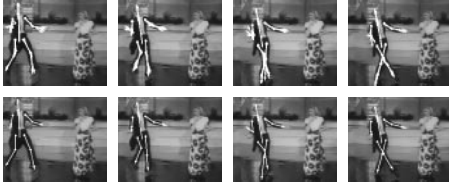
Figure 7: Mode-based Multiple Hypothesis Tracking Results. Top row: the multiple modes of the tracker are shown. Bottom row: the dominant mode is shown, which demonstrate the ability of the tracker to handle ambiguous situations and thus survive the occlusion event.
