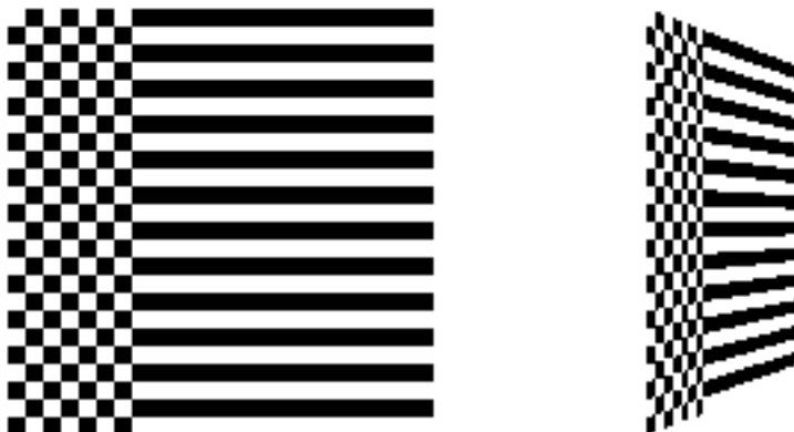
Figure 9-9 Repeating and Clamping a Texture
