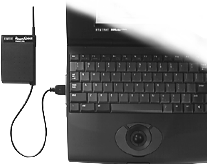
RoamAbout 2.4 GHz Frequency Hopping (FH) PC Card in Digital's HiNote PC
