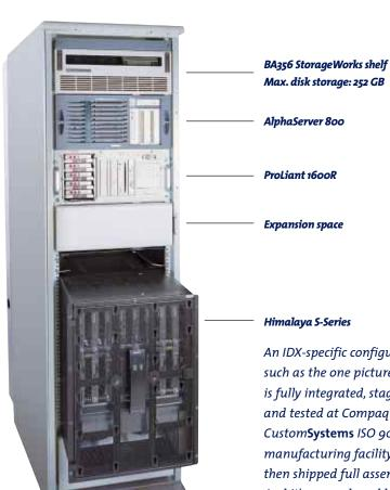
An IDX-specific configuration such as the one pictured here is fully integrated, staged, and tested at Compag Custom**Systems** ISO 9001 manufacturing facility and then shipped full assembled. And it's covered worldwide by industry-leading Compag service and support.
