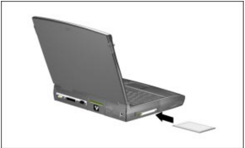
Inserting a PC Card
