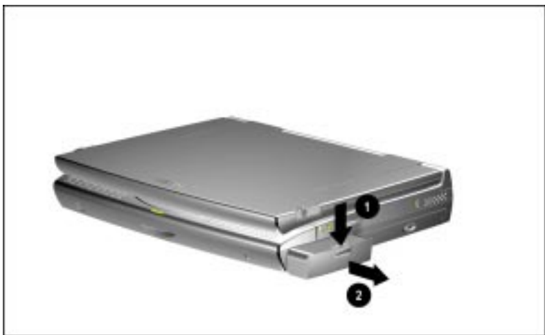
Removing Battery From Battery Bay
