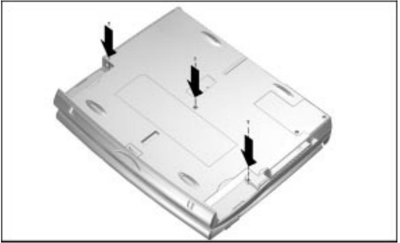
Reinserting the Bottom Screws
