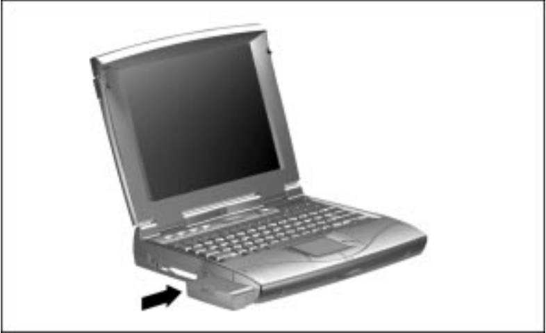
Inserting a Battery Pack into the DualBay
