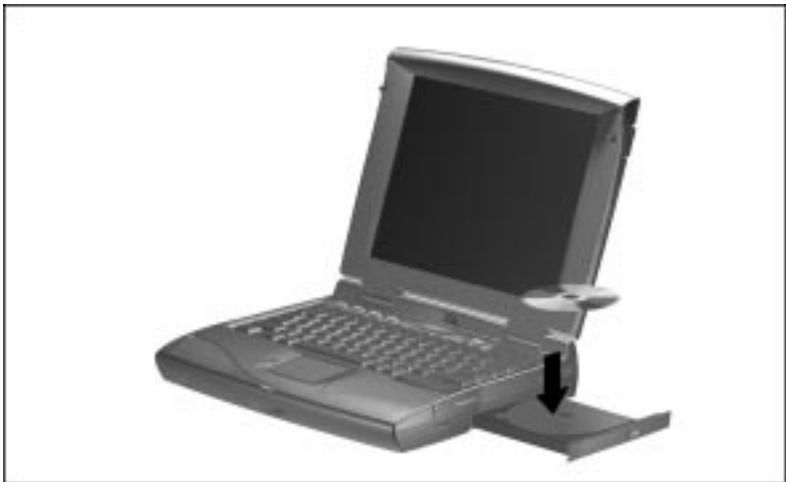
Inserting a CD-ROM Disc
