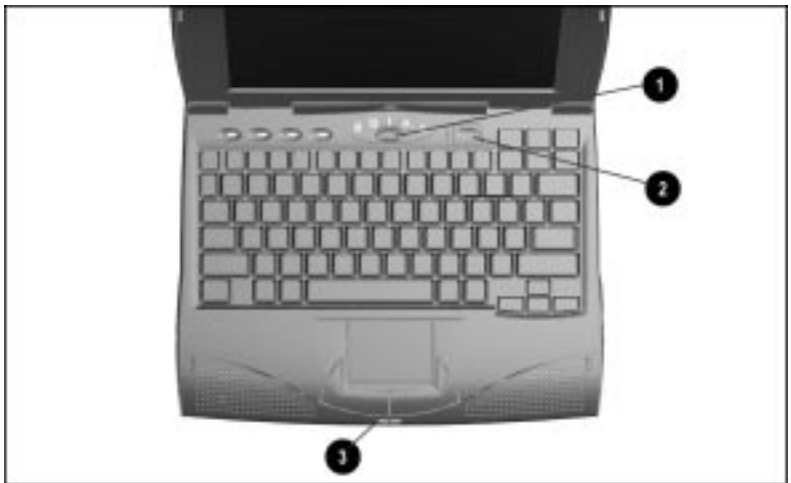
Suspend Button, Power Switch, Power/Suspend Light
