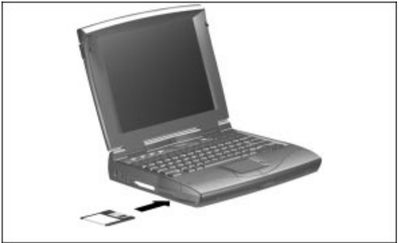
Inserting a Diskette into the Diskette Drive
