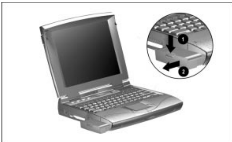
Removing a Battery From the DualBay
