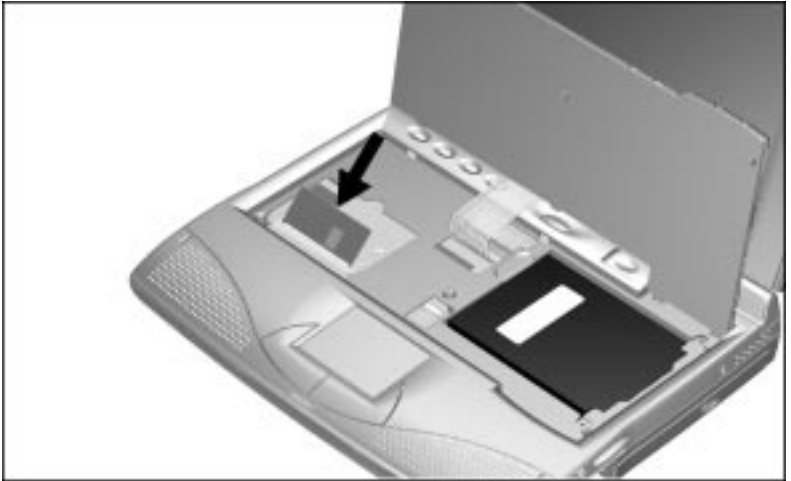
Installing the Memory Board
